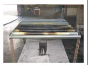
The top surface of the SL Fire Retardant achieved a peak temperature of 652.7°C and was reached at 265 seconds as the sheeting became engulfed in flames.
